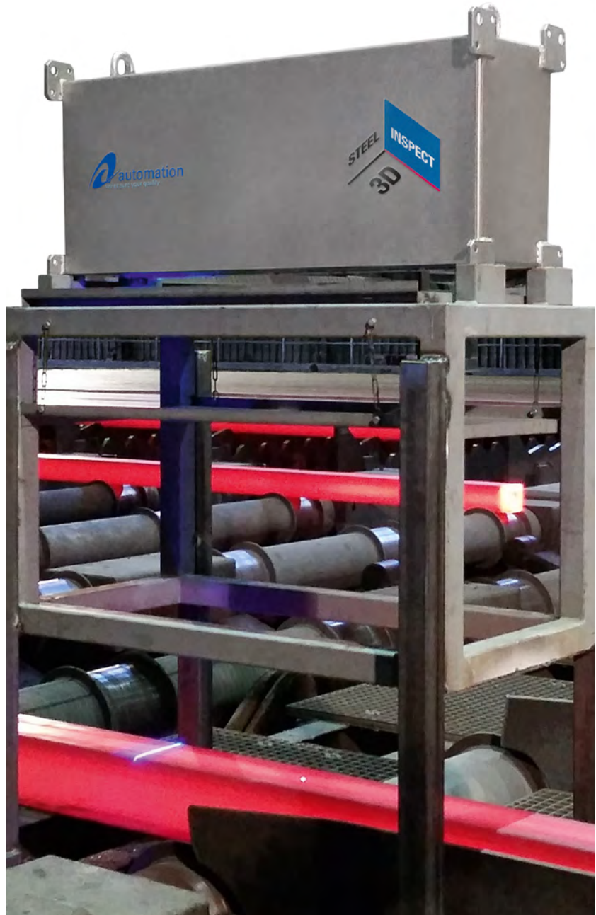
Inspection of a billet while it is about to leave the continuous caster
