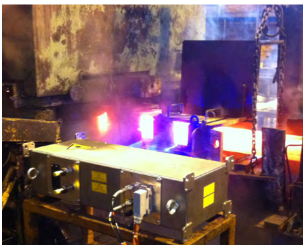
Steelinspect 3D Measuring Head, Lateral Installation in a Rolling Mill.
